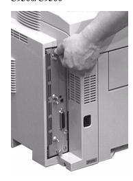
4. Grasp the control board, loosen it by wiggling it back and forth, and slide it out of the printer.
